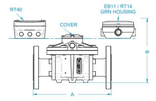
OM040: Ø6.3 in. (160 mm) OM050: Ø7.1 in. (180 mm) OM015: Ø4.3 in. (110 mm) OM025: Ø4.7 in. (120 mm)
